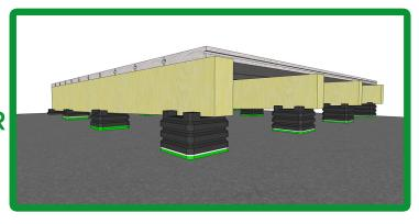
Stacked on top of each other and packed with our packers to level out angled surfaces
