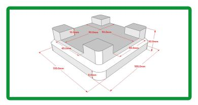
The versatile design allows it to be used with both 45mm and 50mm wide timber joists.
